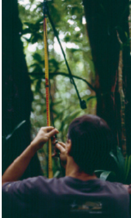
Dr Reillo prepares the peeper video camera system. The small camera, mounted on the end of the adjustable boom is used to monitor inside nest cavities using the telescoping pole to which it is attached.
